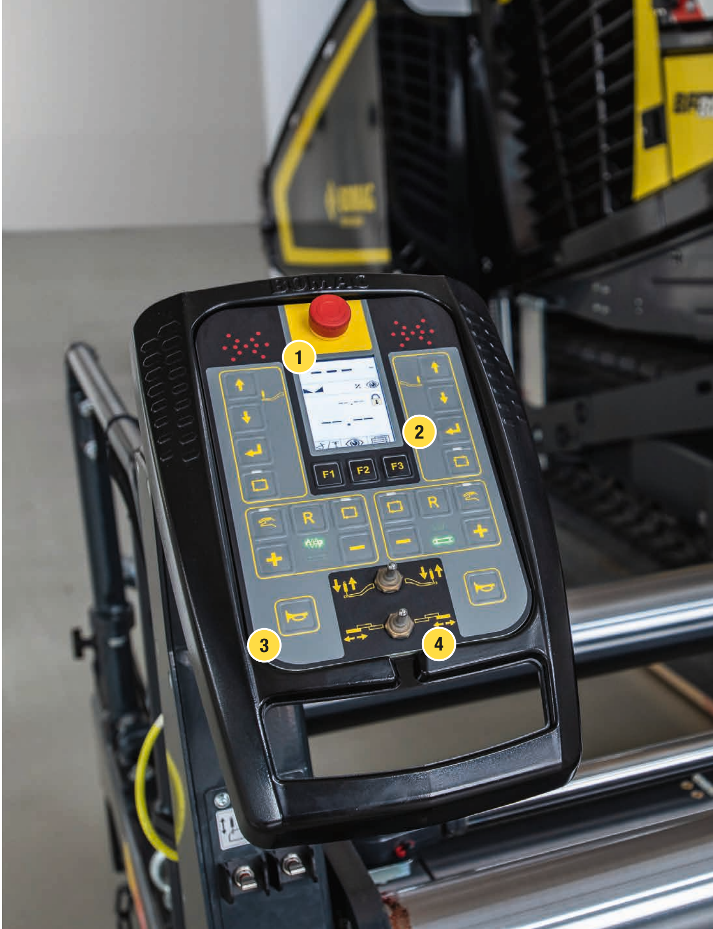
The side-mounted control panel provides exactly the information that is crucial for paving.
