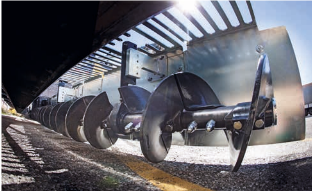
400 mm auger made of wear-resistant cast iron.
