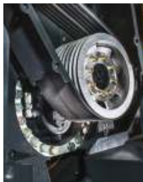
With external cooling and filtration of gear oil, the milling gear is highly robust.
