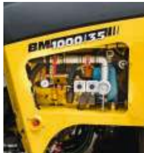
The water system can be accessed easily and, due to the clearly arranged components, is quick to service.
