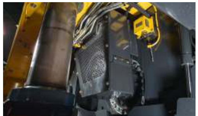
Crawler tracks and lift posts are of solid design. The extra diameter of these posts reduces area contact pressures and prolongs the life of the guides.
