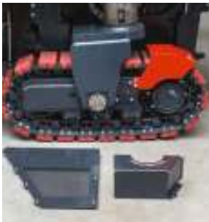
The power belt cover is divided into two parts for servicing by one person.
