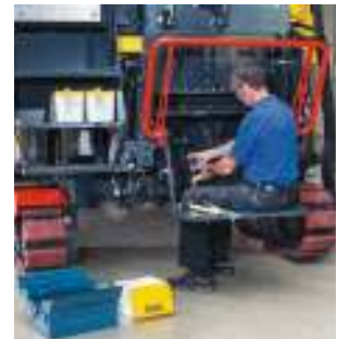
Large stowage compartments for tool boxes close to service locations.
