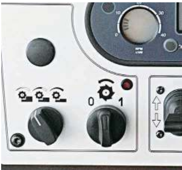
Manually adjustable - best cutting speed for any application.
