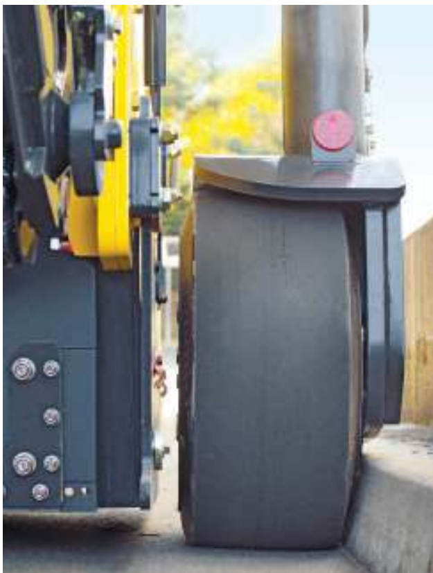
Ultimate ground clearance due to optimised gear housing.
