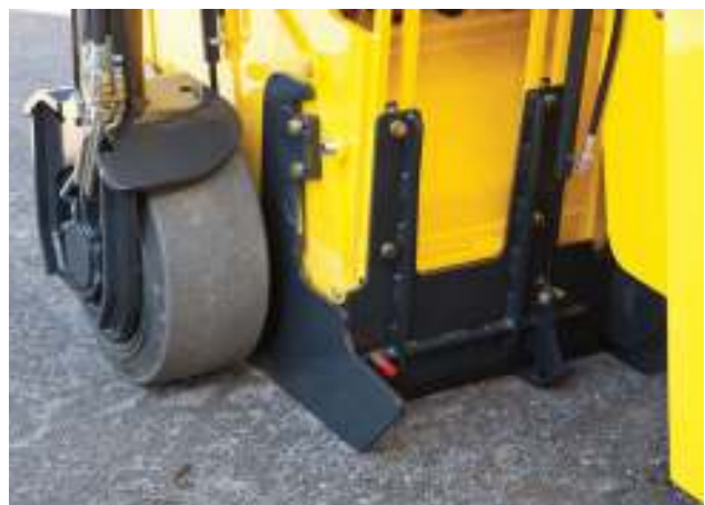
Hard metal grade shoes – they can withstand a lot of wear.
