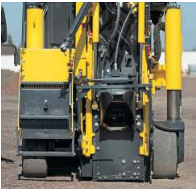
Optional – the split design scraper door.
