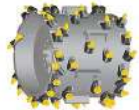
Quick-change milling drum Milling width: 600 mm Line spacing: 15 mm Milling depth: 0-210 mm
