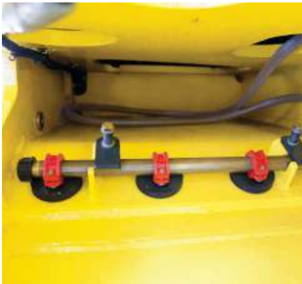
The water spray bar can be easily accessed and ...
