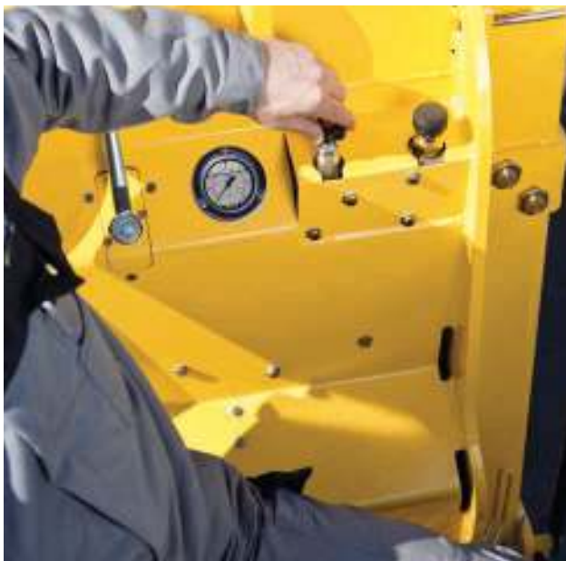
Convenience while seated – adjusting the scraper pressure.
