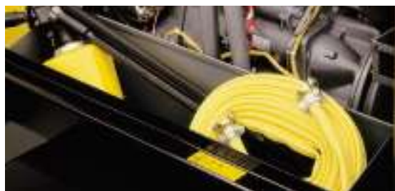
Pneumatic equipment such as hoses and breakers can easily be locked away inside the canopy if no generator is installed.
