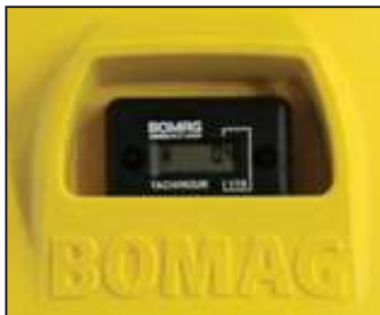
Easy service: hour and rpm meter with integrated service indicator.
