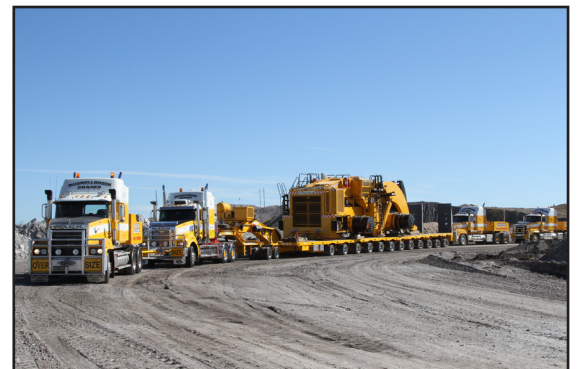
Above - Professional synchronisation between drivers was critical to the smooth and safe hauling of the load
