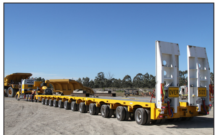
Above - Drake semi modular 12 line low loader. This 12 line loader consists of 3 sections, 1 X 2 line, 1 x 3 line and 1 x 7 line trailers
