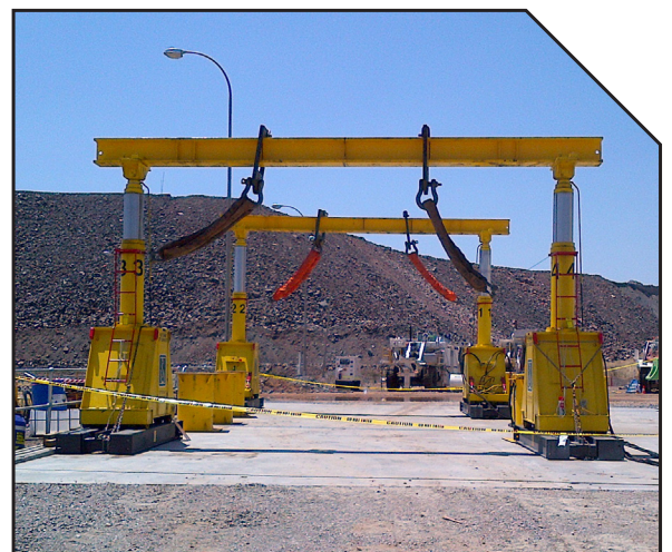
Above - Tutt Bryant's 4 Point Lift Jacking System
