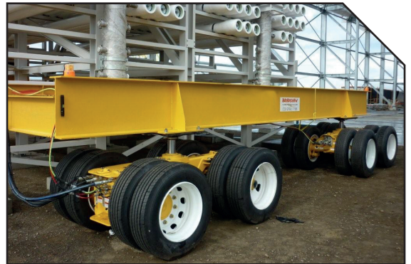
Above - The Power Dollies feature power steering and free-wheel hydraulic drive on the 2 power dollies for improved manoeuvrability.
