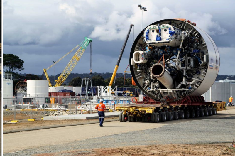
Left: Sourced from: https://www.metronet.wa.gov.au/projects/forrestfield-airport-link ; Right: TBHL&S SPT crew moving TBM Sandy's Front Shield Unit
