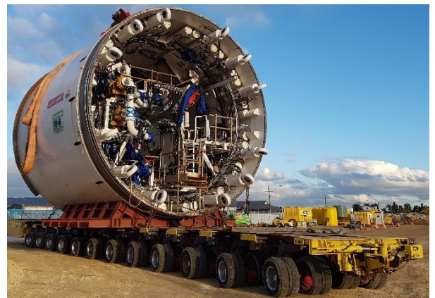
Above: TBHL&S Self-Propelled Trailer transporting TBM Grace's Middle Shield to the dive site in Forrestfield
