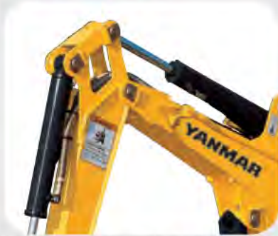
* [P.T.O. specification] VBE : Attachment pipe on the boom end
