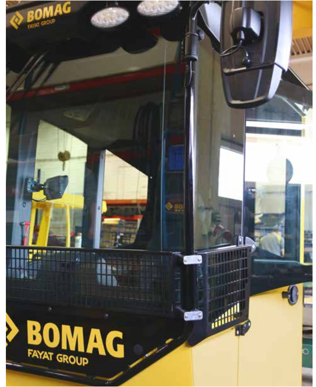
Cab protection grille protects damage to the cab windows.
