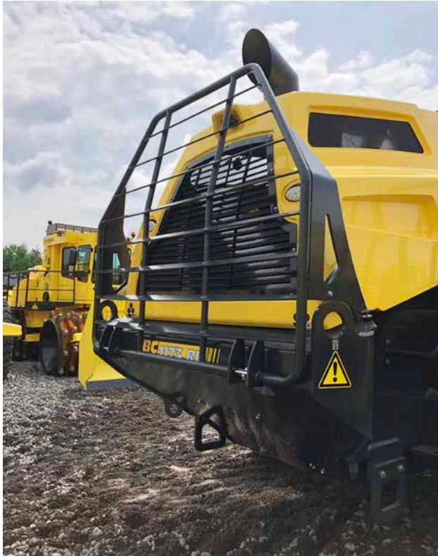
Rear bumper protects the rear of the bonnet from damage.
