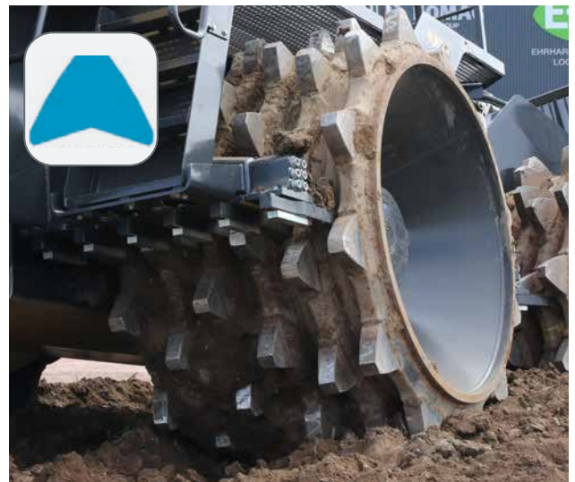
BOMAG wheels with weld on teeth.
