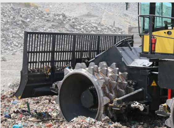
Scrapers ensure clean wheels and high compaction.
