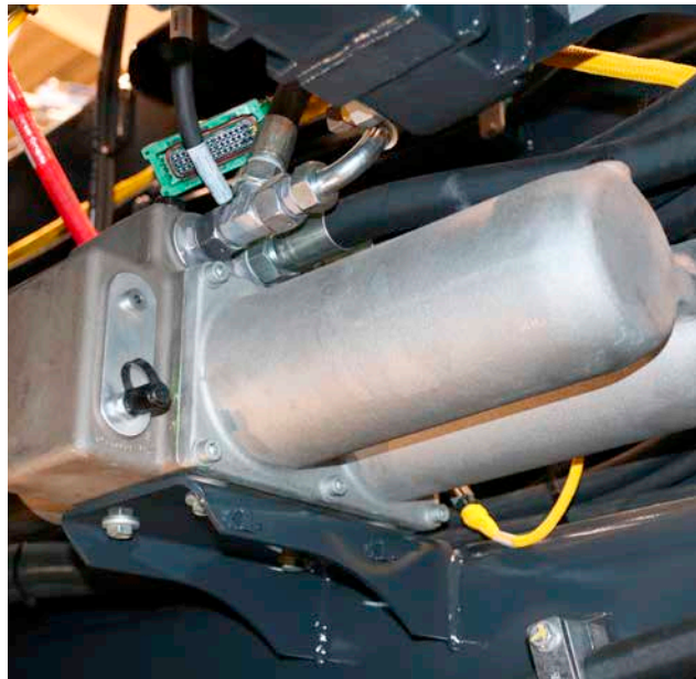
Electronic monitoring of hydraulic return filter.
