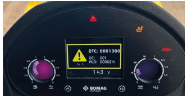
Diagnostic interface with error code shown on the display.
