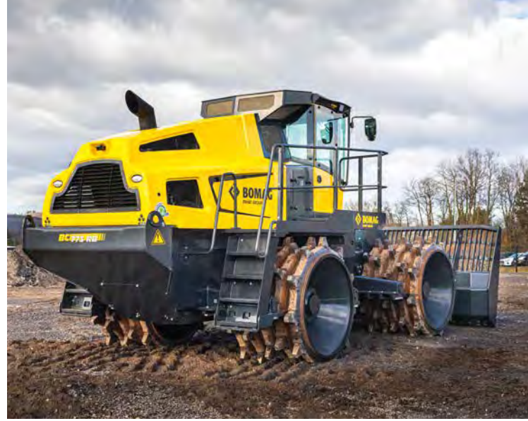
The service platform provides access to the maintenance area.
