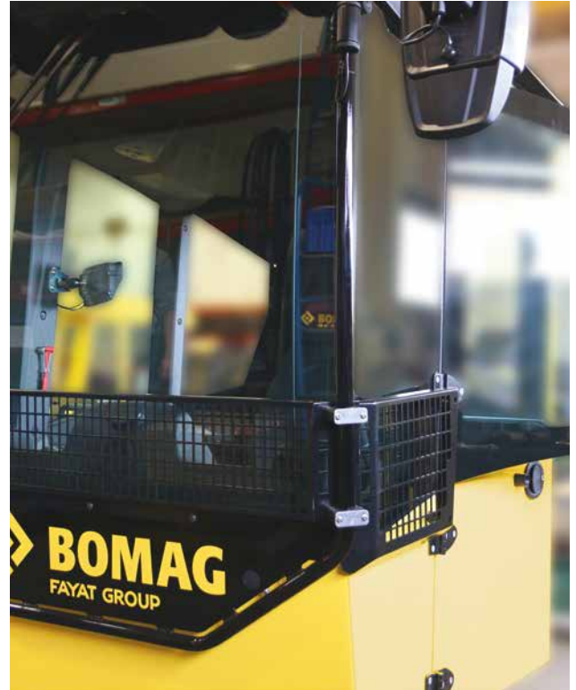
Cab protection grille prevents damage to the cab windows.
