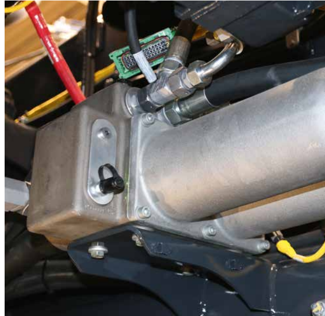
Electronic monitoring of hydraulic return filter.
