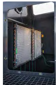
Access to the radiator and maintenance opening for the air conditioning unit.
