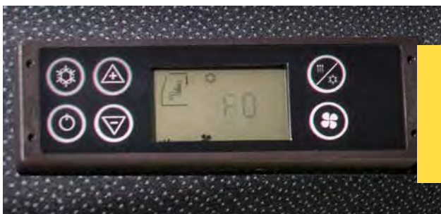
Automatic heating and air-conditioning unit control panel.
