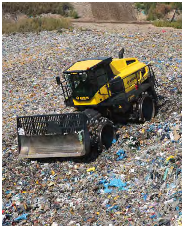
Optimum compaction with the oscillating joint, providing good load distribution to the compaction wheels.
