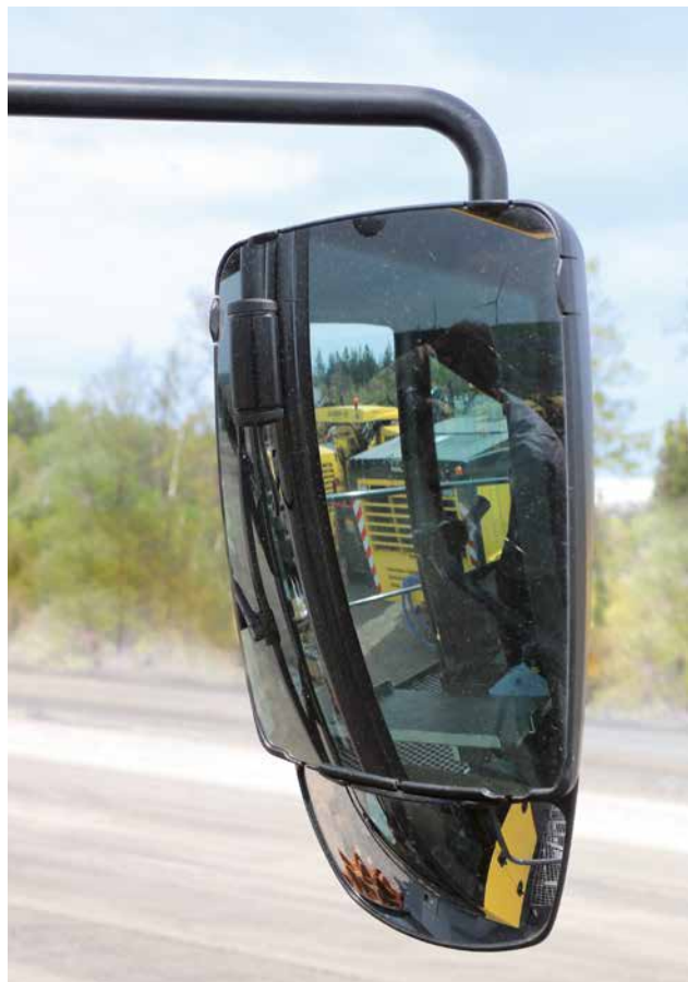
Mirrors optimally adjusted due to electrical regulation.
