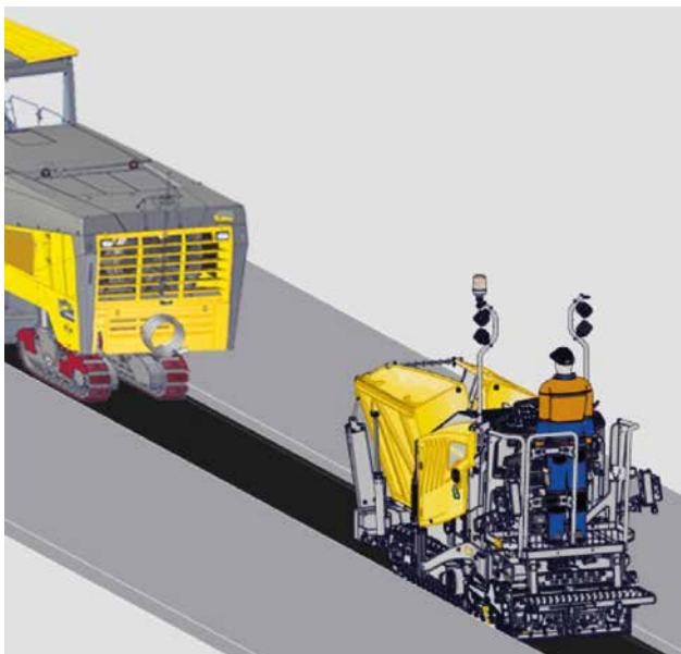
The BF 200 C-2 is in its element for paving widths of 1.1 m and above.
