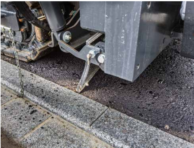
Chain scrapers guarantee low maintenance.
