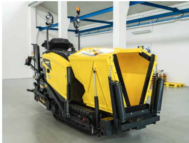
Long crawler tracks ensure dead straight paving.
